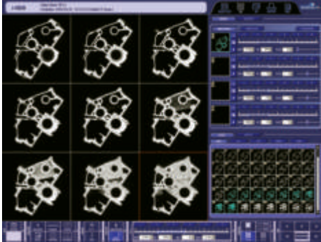
2D CT images of a V8 Engine in i-view Workspace.
